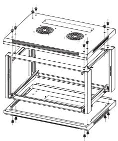
(2) Install the vertical rails by 8pcs M6\*12 screws and 8pcs M6 cage nuts
